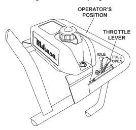
Figure 11. Throttle Lever (Full Open)
